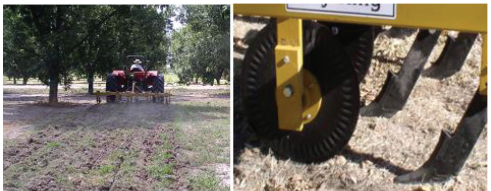
Fig. 3. Minimum-till surface chisels used for improving soil permeability.
