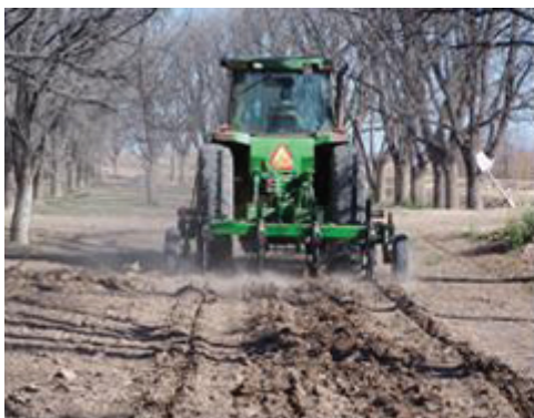
Fig. 5. Subsoilers used for improving soil permeability.
