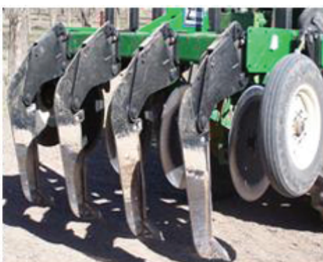
Fig. 5. Subsoilers used for improving soil permeability.
